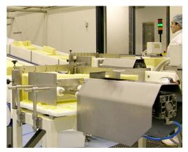
The operator can access remotely the system of checkweighters and verify the weight of the product instantaneously
