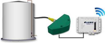
The Netbiter Ultrasonic Tank Sensor detects the fuel level with less than 1% error margin. The Netbiter gateway sends data via the cellular network to Netbiter Argos...
