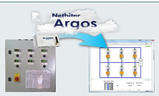
In the brewery control panel (left), it is possible to see all current values in the system. A Netbiter gateway is connected to this control panel and sends data to the Netbiter cloud service which can be accessed at www.netbiter.net (right). Here, the users can see the same thing online as the can in the real panel. The brewery can also control the equipment and get alarms if a value reaches a certain level.
