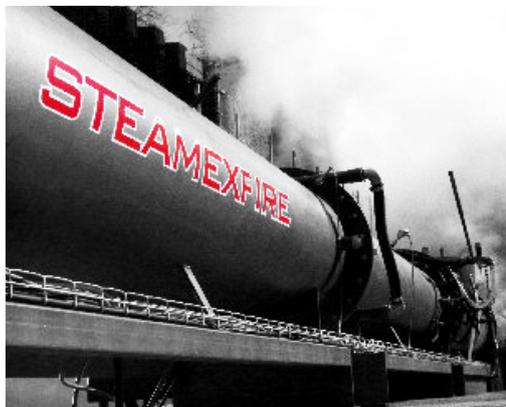
The heart of each Steamexfire is a jet fighter turbine producing enormous quantities of oxygen-free steam. This steam can be used to put out fires in large enclosed spaces
