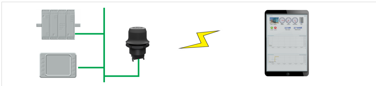
Fig. 1 Accessing a PLC from a handheld device using WLAN
