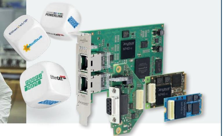
*Ixxat INpact is available in three form factors: PCIe, PCIe Mini and M.2 card – enabling implementation in industrial PCs, desktop PCs or in mobile devices.*
